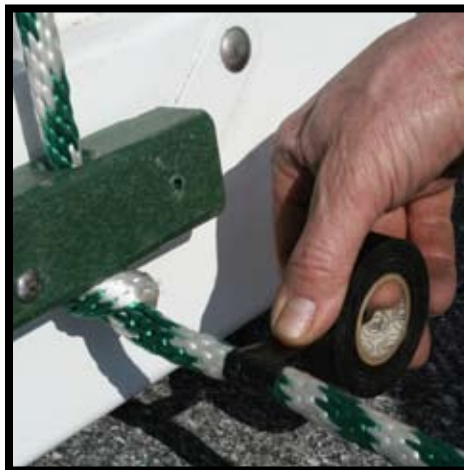
If the rope is too long, wrap tightly with black tape. Then with a utility knife, cut into the tape to separate the excess rope.
