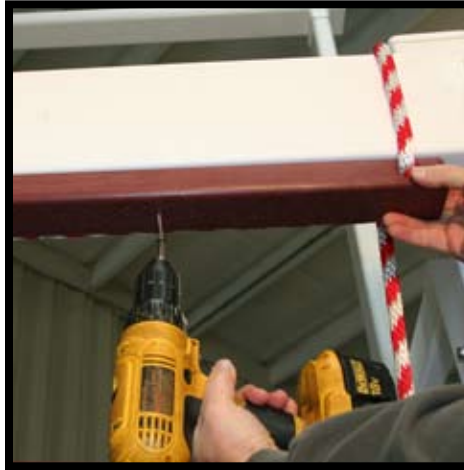
Fasten rope ladder to the activity arm as shown using #8 x 3" square drive stainless steel screws.
