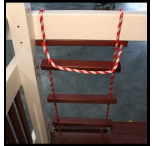
Pull rope back and feed ladder down through as shown.
